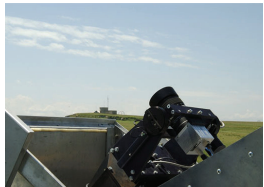
FIGURE 5: MASTER very wide-field camera.
